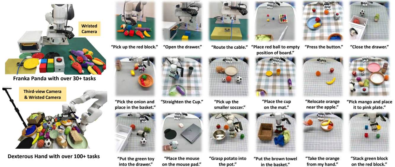
Figure 7. Two real-world hardware platforms and visualizations of sampled tasks. In the Panda arm platform, our experiments include 30+ tasks of 6 categories. In the Xhand dexterous platform, our experiments include 100+ tasks of 10 categories.
